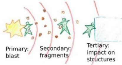
Figure 29: Hazards emanating from an explosion
