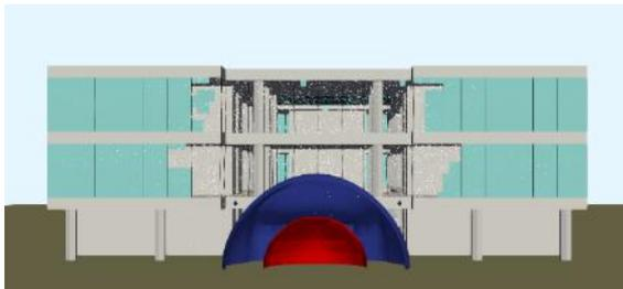
Distance: 25 m. Blue: zone of ear drum rupture; red: zone of 50 % fatality; damaged glass more localised because of short distance of blast from the building.
