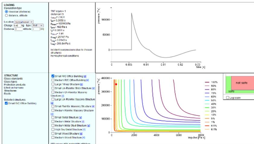
Figure 27: Example from the BIAStool for the calculation of peak pressure / impulse parameters and comparison with pressure–impulse iso-damage curves
