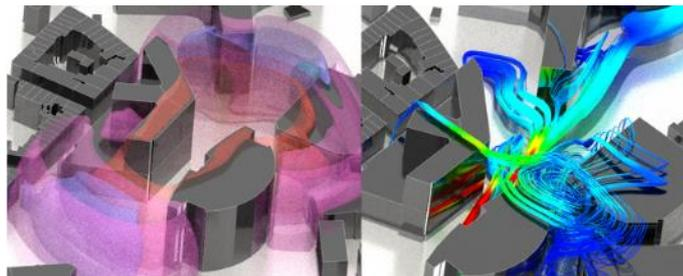
Figure 28: Example from a blast simulation using Europlexus – pressure wave and air flow in an urban environment
