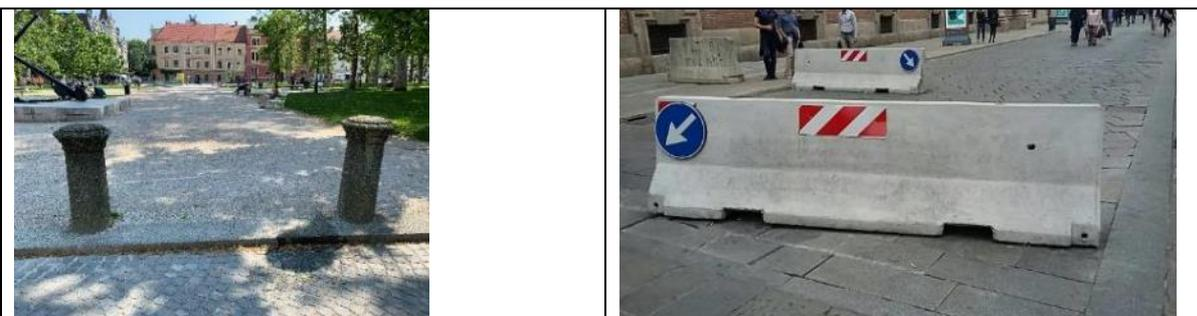
Figure 21: Permanent (left) and temporary (right) barrier solutions
