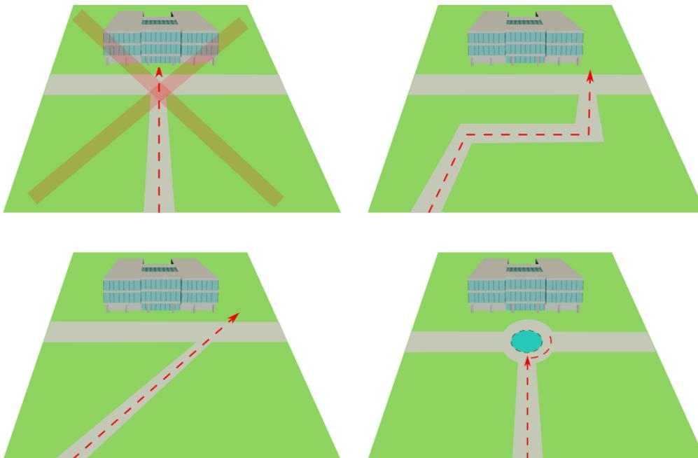
Figure 19: Different speed reduction methods: chicanes (to avoid direct attack approach routes) and indirect access to a site. Source: Inspired by CPNI (2014).
