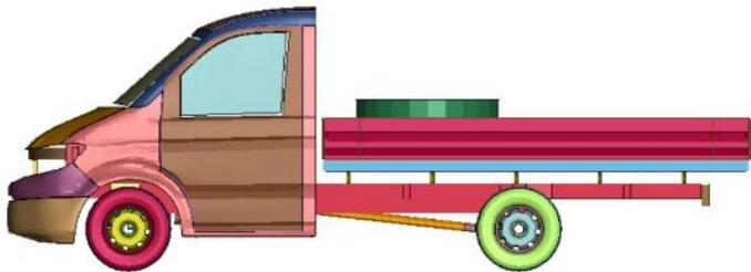
Figure 24: Example of a N1 vehicle simulation model
